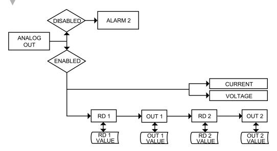
Figure 3.6 Flow Chart for Analog Output (Retransmission)
